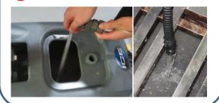
3 DRAIN AND CLEAN SOLUTION TANK
