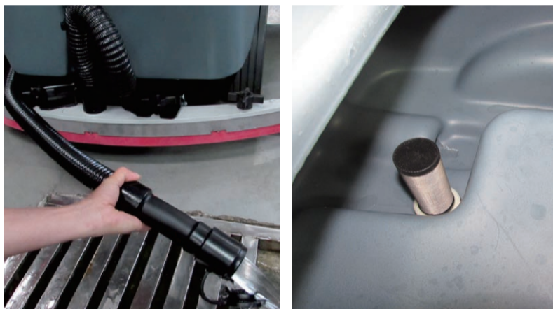
Drain and Clean the Solution Tank, Inspect and Clean the inline Filter Screen Monthly
