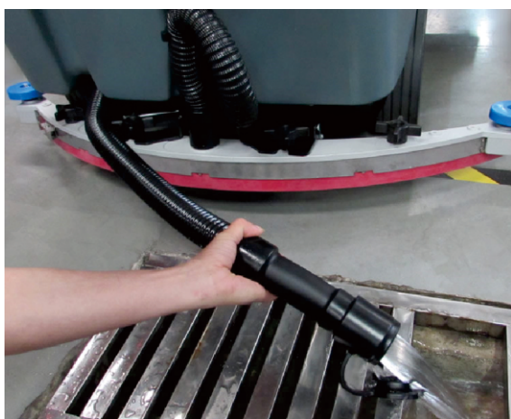
Drain and Clean Solution Tank
