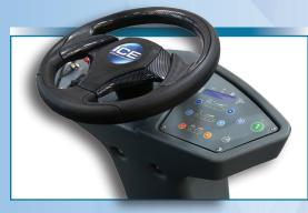
Intuitive, state-of-the-art control panel and a programmable switch to set brush pressure, solution flow, and chemical mixing ratio
